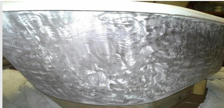
**Using a flapper grinder we remove the high spots in the metal casting.**
